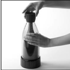
Fig. 9: Screw cap on with gentle force
